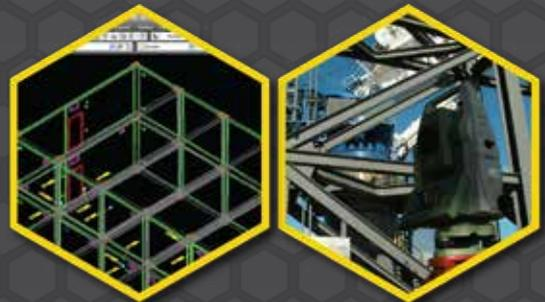
Dimensional control can be defined as the process of acquiring accurate dimensional information that is spatially referenced to a known or established benchmark. Using the latest survey technology from Leica Geosystems, 3B's surveyors can measure and produce 3D CAD models from single pipe spool replacements to full FPSO / Jacket construction surveys.
