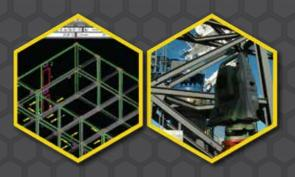
Dimensional control can be defined as the process of acquiring accurate dimensional information that is spatially referenced to a known or established benchmark. Using the latest survey technology from Leica Geosystems, 3B's surveyors can measure and produce 3D CAD models from single pipe spool replacements to full FPSO / Jacket construction surveys.
